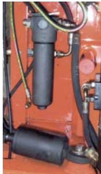
[above] FMP - Pressure line filter with A10 - Beta 200 element media fitted
